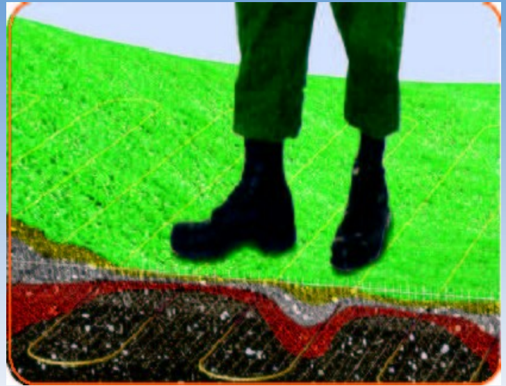
RLTD Fiber Sensor can also be buried for invisible perimeter intrusion detections.
