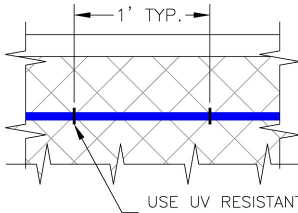
USE UV RESISTANT TIE WRAPS TO SECURE THE FIBERGUARD CABLE TO THE FENCE. DO NOT OVERTIGHTEN THE TIE WRAP AS TO PINCH THE CABLE.
