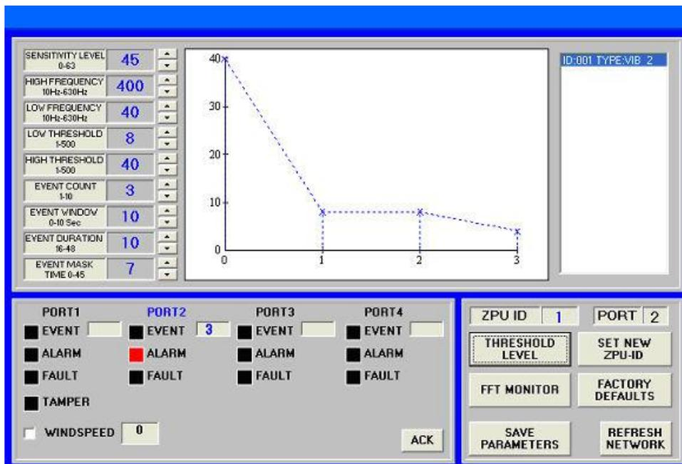
By adjusting the sensitivity, frequency, and thresholds the graph gives the user a representation of the fiber activity in quiescent or an intrusion state.
