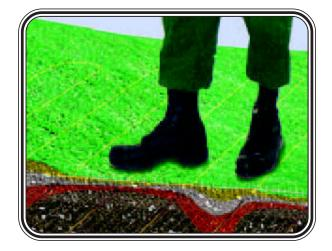
The **FiberSensor XL** buried sensor system is comprised of fiber-optic cables buried across a wide horizontal plane. The system detects pressure applied on the ground above the cable. The buried sensor cable is invisible, completely passive, and can be installed in almost any ground.
